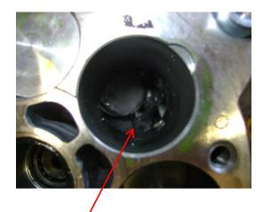
Metal particles in the Piston shaft, where the piston has broken down because no oil was added.
