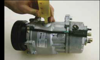
5. Adjust oil quantity according to manufacturer's advice
