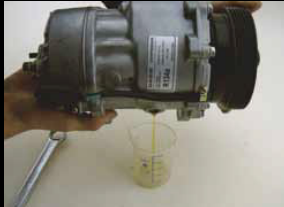
3. Drain compressor completely
