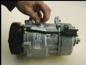
6. Put drain plug back into compressor
