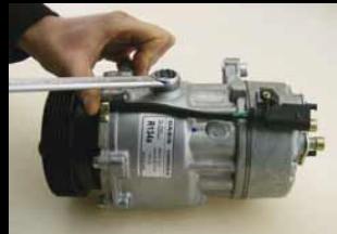
7. Tighten drain plug (but DO NOT over tighten)
